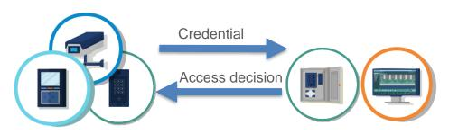
**Input device** (e.g., token readers, biometric readers, cameras, keypads, sensors) and **output device** (e.g., locks, displays, LEDS)
