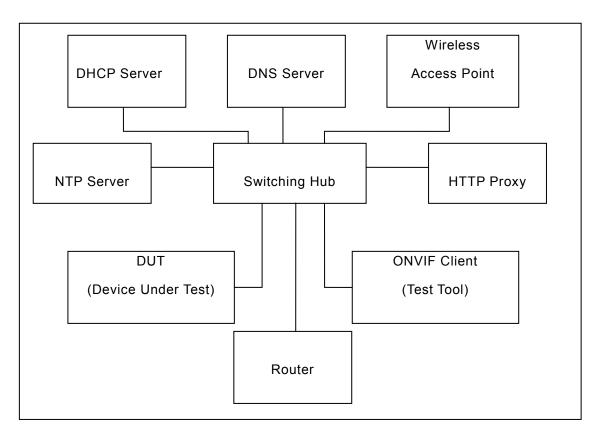
Figure 1: Test Configuration for DUT
