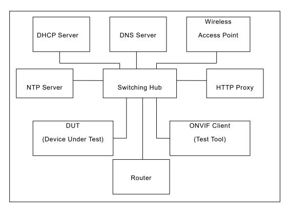
Figure 1: Test Configuration for DUT
